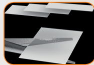
Cut out two or three fibre strips of different widths
